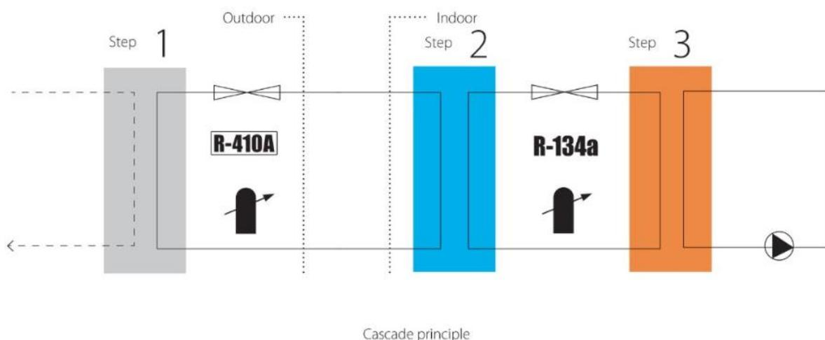
Image 2.1 – Air to Water Refrigerant Cycle
