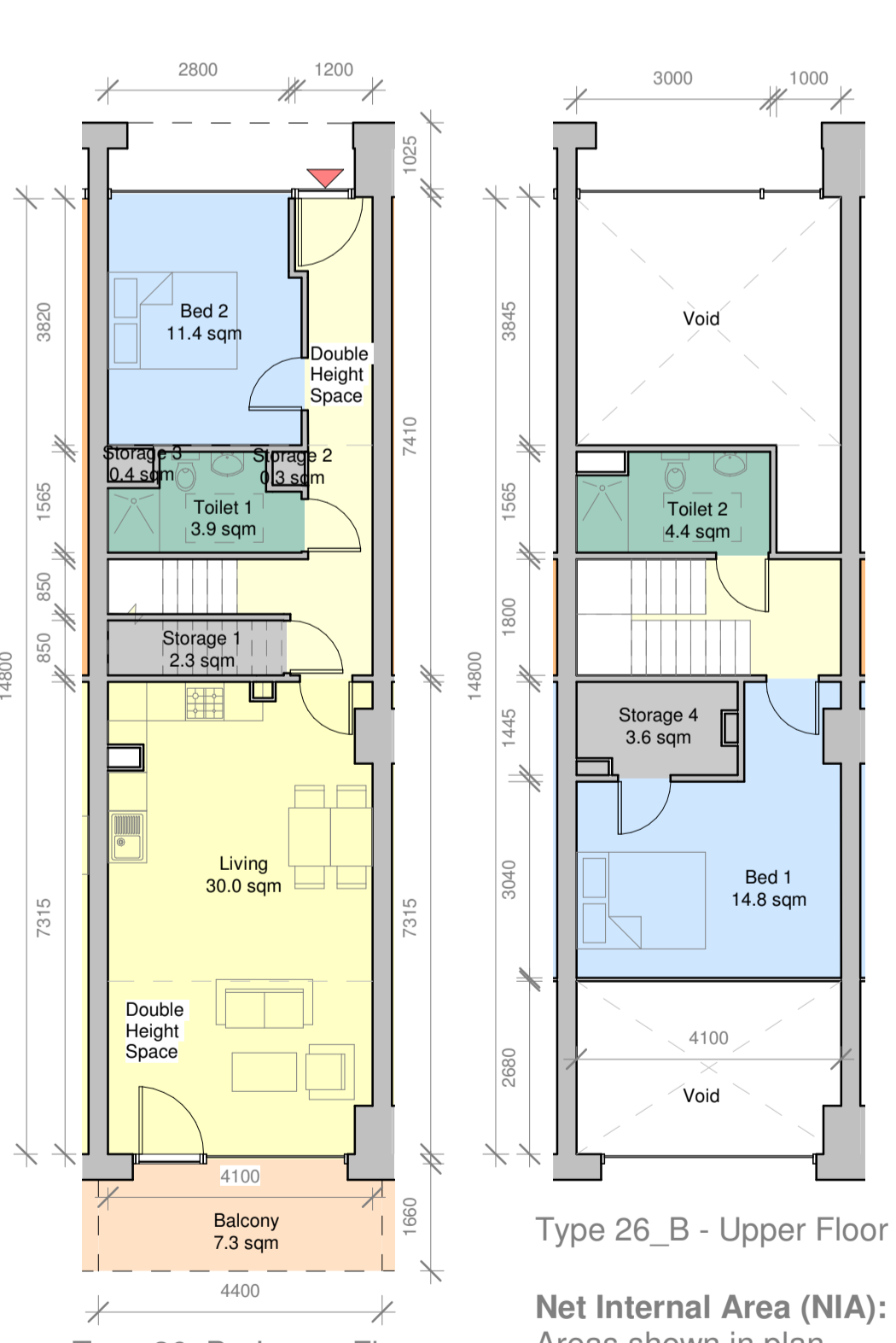
Type 26_B - Lower Floor (Entry Level)
